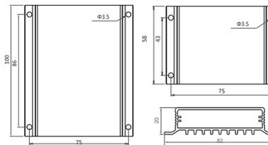
Installation of controller should be stable and dimensions are as follows:
