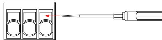
2) The inverter is equipped with a standard American-Standard terminal, as shown in the drawing below, with a maximum current capacity of 20A.
