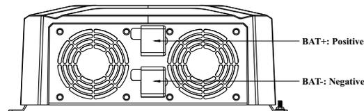
⚠ There is no reverse connection protection for the input, check if the Positive and Negative are connected correctly before connecting, or the inverter may be damaged!
