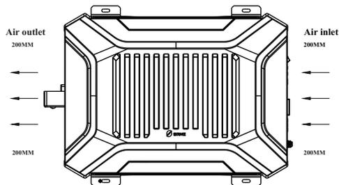
⚠ If the device is installed in a closed box, ensure that heat dissipation is allowed through the container. Otherwise, derate to use the device.
