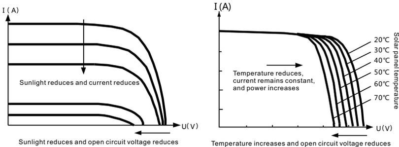
Figure 1-3 Solar Panel Output Characteristic and Lighting Relation
