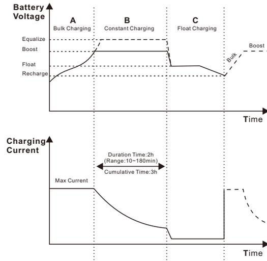
Figure 1-4 Battery Charging Stage
