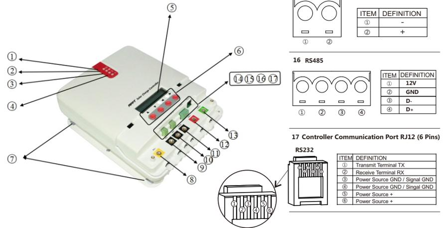
Figure 1-1 Solar Charge Controller Appearance and Interface
