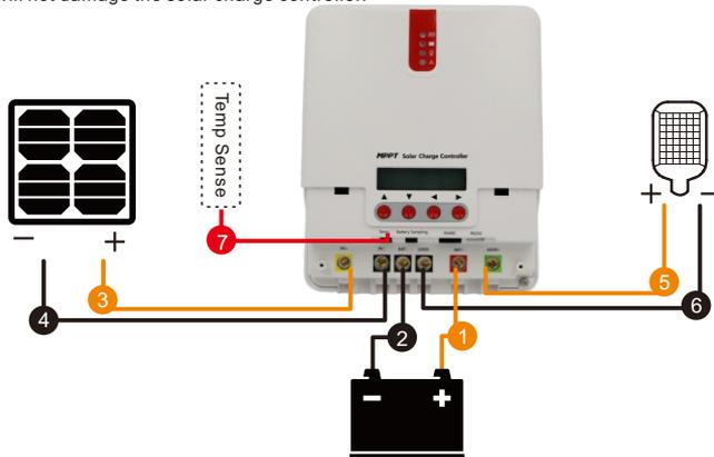
Figure 2-3 Wiring
