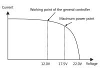
The voltage of the solar panel is about 12V when
