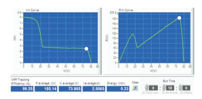
2. There's shadow at the top left corner of PV module, the tracing efficiency is 99.61%.
