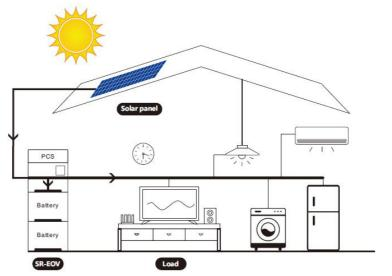
At night, the battery supplies power to the loads through the power module.
