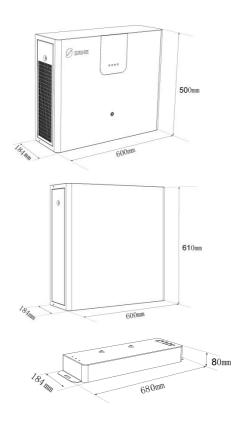
Inverter dimensions (L\*W\*H):600\*184\*500mm Battery dimensions (L\*W\*H):600\*184\*610mm Base dimensions (L\*W\*H):680\*184\*80mm
