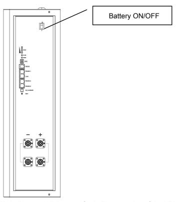
After the power switch is turned on, the LED indicator will light up or flash. The meaning of the LED indicator is as follows.
