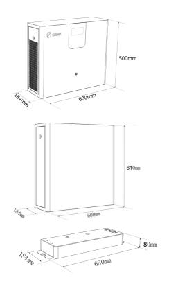
Inverter dimensions ( L\*W\*H ) :600\*184\*500mm Battery dimensions ( L\*W\*H ) :600\*184\*610mm Base dimensions ( L\*W\*H ) :680\*184\*80mm
