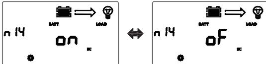
Turn on load short-circuit protection    Turn off load short-circuit protection
