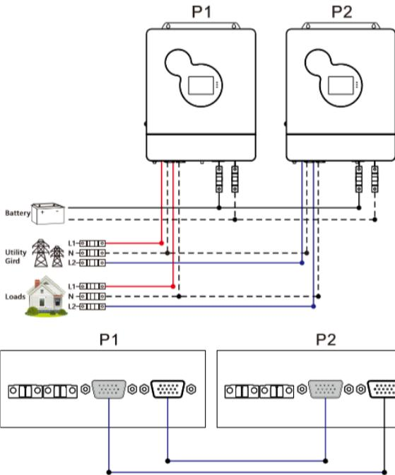
b) Three all-in-one solar charge inverters of the system connected in two phase: 2+1 system:
