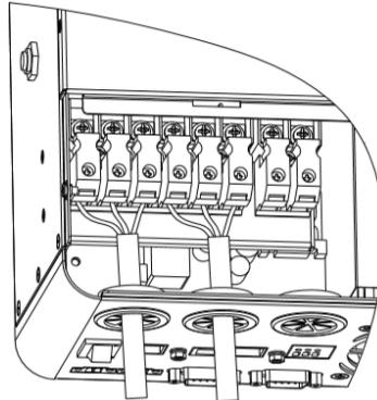
**Note:** The grounding wire shall be as thick as possible (cross-sectional area is not less than 4mm<sup>2</sup>). The grounding point shall be as close as possible to the all-in-one solar charge inverter. The shorter the grounding wire, the better.
