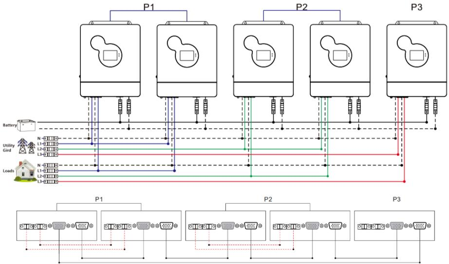
**d) Six all-in-one solar charge inverters of the system connected in three phase:**
