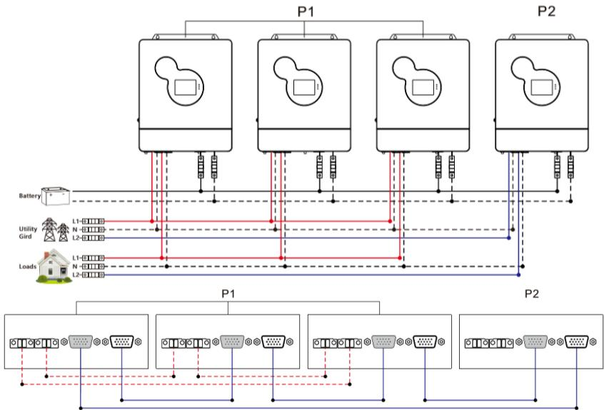
d) Five all-in-one solar charger inverters of the system connected in two phase:
