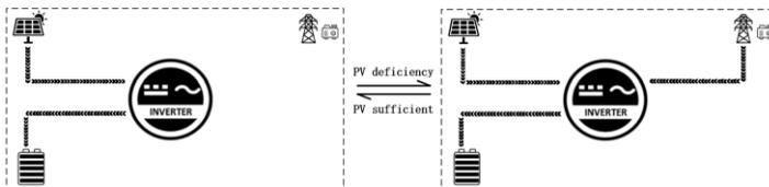
4. **Only Solar:** Only PV charging, no mains charging is initiated. This is the most energy-efficient mode and the battery power comes from solar energy, which is usually used in regions with good daylighting conditions.
