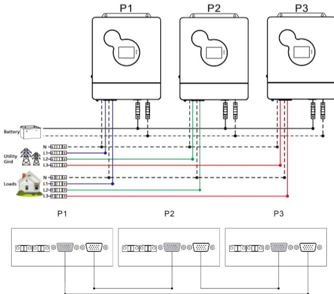
b) **Four all-in-one solar charge inverters of the system connected in three phase:**
