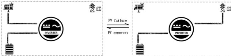
2. **Mains First:** priority shall be given to charging by Mains Power, and charging with PV power will be started only when the Mains has failed.
