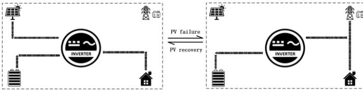
2. **Mains First:** switch to inverter power supply only when Mains Power has failed, which is equivalent to backup UPS and is used in regions with unstable power grid.
