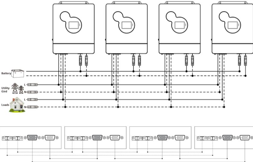
**d) Five all-in-one solar charge inverters of the system connected in parallel:**
