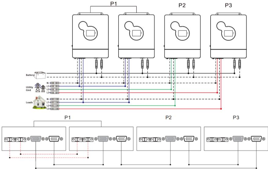
c) **Five all-in-one solar charge inverters of the system connected in three phase: 3+1+1 system:**
