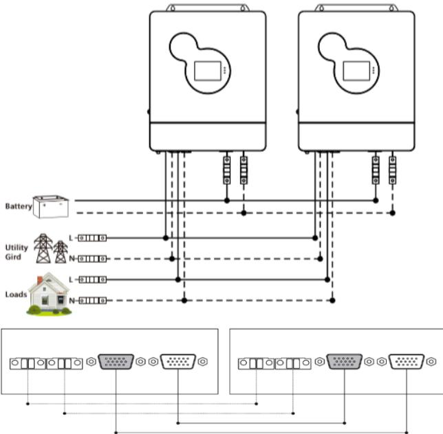
**b) Three all-in-one solar charge inverters of the system connected in parallel:**
