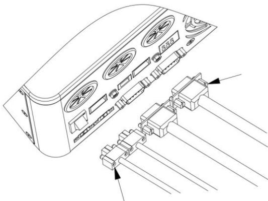
2. In case of parallel operation with multiple inverters, the schematic diagram of parallel connection is as follows:
