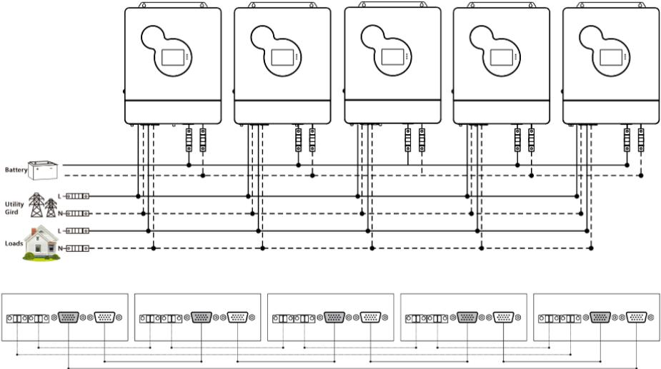
e) **Six all-in-one solar charger inverters of the system connected in parallel:**
