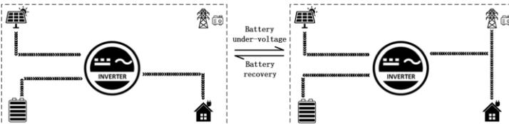
4. **Hybrid output and grid connection (need to be able)** In the utility bypass state, when no battery is connected or when the battery is full, the load power is supplied by the PV and the utility together if the hybrid function is enabled, and the surplus PV energy is fed back to the grid if the grid connection function is enabled.
