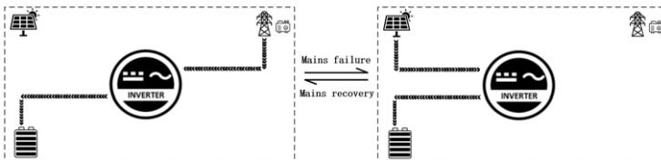
3. **Hybrid Charging:** hybrid charging of PV and Mains Power, give priority to PV MPPT charging, and supplement Mains Power when PV energy is insufficient. When the PV energy is sufficient, the Mains Power will stop charging. This is the mode of fast charging and suitable for unstable areas of power grid, and can provide sufficient backup power at any time.
