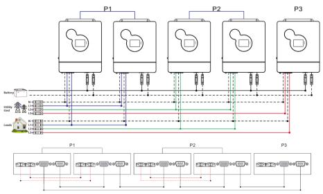
d) Six all-in-one solar charger inverters of the system connected in three phase:
