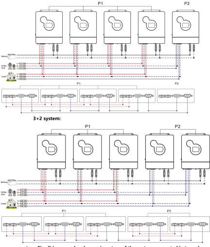
e) Six all-in-one solar charger inverters of the system connected in two phase:
