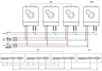
d) Five all-in-one solar charger inverters of the system connected in two phase:4+1 system:
