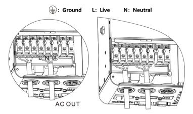
**Note:** The grounding wire shall be as thick as possible (cross-sectional area is not less than 4mm<sup>2</sup>). The grounding point shall be as close as possible to the all-in-one solar charge inverter. The shorter the grounding wire, the better.
