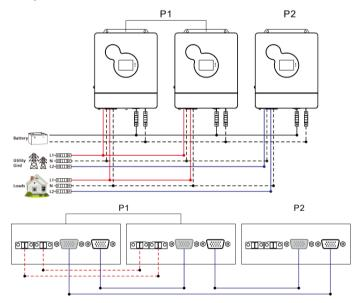
c) Four all-in-one solar charger inverters of the system connected in two phase:
